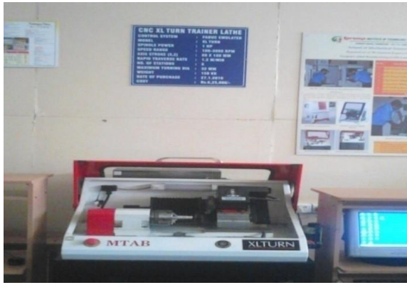
Fig. 1. Experimental set up using XLTURN- CNC lathe
